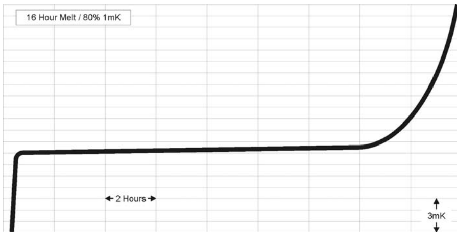
Graph 5: Siphonic Zn Fixed Point Cell Melt Plateau (24 th February 2009)
