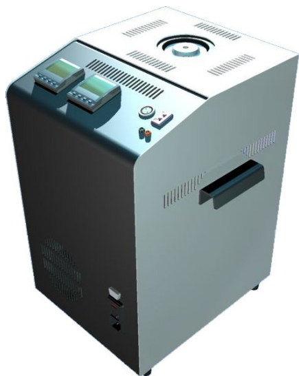
Figure 2: ITS-90 Isothermal Tower
