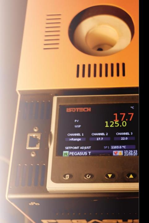
Fully featured high resolution display with advanced control features including multi loop control with autotune, adjustable temperature alarms with control from internal or external thermocouples
