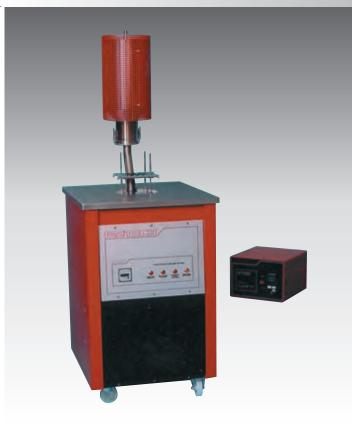
temperature stability and uniformity cannot be achieved in the fluidized medium itself. They are obtained by using large metal blocks or by inhibiting the fluidizing action in the powder around the work piece - either locally, or by completely collapsing the bed at the required temperature, this is not the case with the 875. A full evaluation report is available upon request. The bath is fully commissioned, tested and charged with the correct amount of aluminium oxide powder before despatch.
