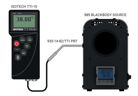
Model 989 features a reference thermometer pocket that is located in the blackbody block just below the surface. If desired a calibrated platinum resistance thermometer can be added for traceability. Isotech can provide either ISO 17025, UKAS Calibrated Model 938-14-82/TTI Semi Standard Thermometer or TTI-10 High Accuracy Digital Readout with a Model 938-14-82/TTI Thermometer, UKAS Calibrated, Uncertainty 0.02°C, 20mK.
