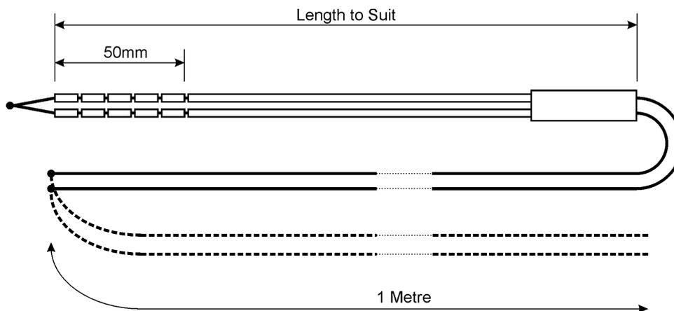
0.1 to 0.2mm  $\tau$  type R thermocouple wire with Alumina insulators  $5 \times 10\text{mm}$  long by 0.9mm outer diameter on each wire. Then two longer insulators to make a total hot length of 200mm. The thermocouple was made continuous for a further 1 metre and insulated in kapton to two cold junctions where the Type R wire was connected to two copper multi strand Teflon insulated wires 1 metre long to load the signal to a DVM.
