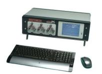
The microK includes a graphing facility with auto or configurable scales. It can also log the data to its internal memory or plug in a USB Pen Drive and log directly to that.
