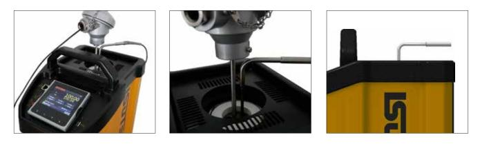
Termination Options Bare Wire (BW) DB Connector for Dry Block Calibrator Site Indicator
