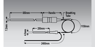
Economic alternative to HTSPRTs Construction allows for differential expansion Accuracy of ±0.05°C over the whole temperature range
