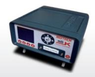
The milliK is a very high accuracy thermometer - capable of performance to 0.003°C with SPRTs and PRTs and also enables high accuracy measurement from thermistors, thermocouples and even 4-20 mA process inputs. It can be expanded to have up to 33 flexible inputs.
