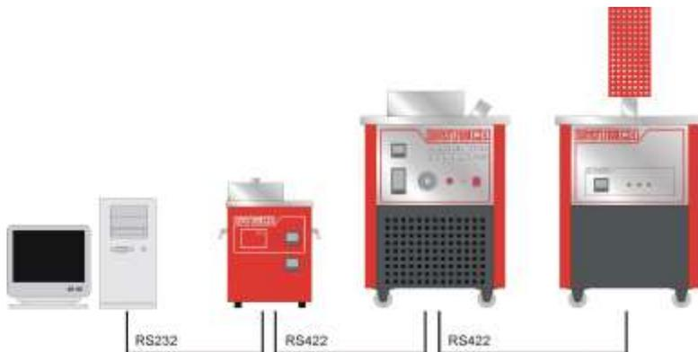
Note: The RS 422 standard specifies a maximum lead length of 1200M (4000ft). A true RS422 port will be required to realise such lead lengths. The Isotech conversion leads are suitable for maximum combined lead lengths of 10M that is adequate for most applications.
