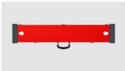
1 Once the SPRT is safe within the carrying case a foam end piece is placed over each end.
