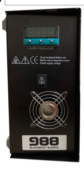
Model No. 988 20°C to 45°C Temperature (70°F to 115°F) Range ±0.1°C Resolution **Target Size** 70mm diameter Greater than 0.97 ± 0.02 **Emissivity** ±0.2°C Combined Accuracy / Stability  $(\pm 0.3^{\circ}F)$ 70W Power 12 V.D.C. Voltage **Dimensions** Height 230mm Width 225mm Depth 115mm Weight 4kg Accessories Switch Mode Power Supply Supplied as Standard How to Order 988
