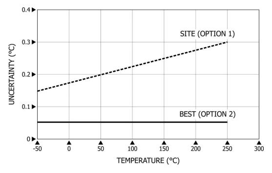
Best uncertainty – using Basic model with a TTI-2 and a 935-14-82 calibrated system Site version uncertainty – Site model using built in indicator at the time of calibration
