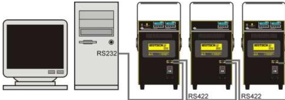
Note: The RS 422 standard specifies a maximum lead length of 1200M (4000ft). A true RS422 port will be required to realise such lead lengths. The Isotech conversion leads are suitable for maximum combined lead lengths of 10M that is adequate for most applications.
