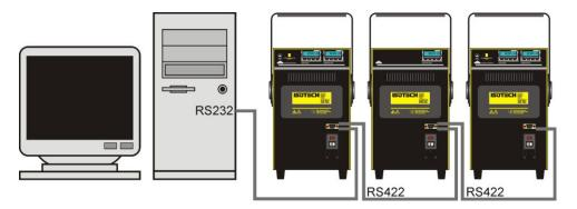
Note: The RS 422 standard specifies a maximum lead length of 1200M (4000ft). A true RS422 port will be required to realise such lead lengths. The Isotech conversion leads are suitable for maximum combined lead lengths of 10M that is adequate for most applications.
