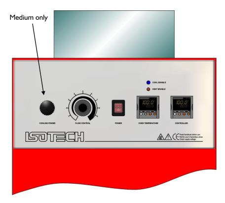
Cooling Power and cool enable are only present on the Orion M model.
