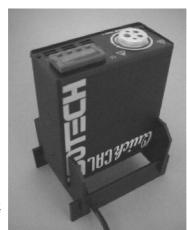
The photo on the right shows the correct position of the Quick-Cal stand.
