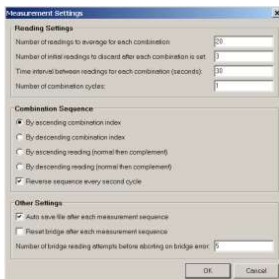
Figure 4.2: The Measurement Settings dialog box showing options for managing the acquisition and averaging of bridge readings, and the RBC combination sequences.
