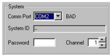
**Comm Port:** Select the serial communication port the instrument is connected to.
